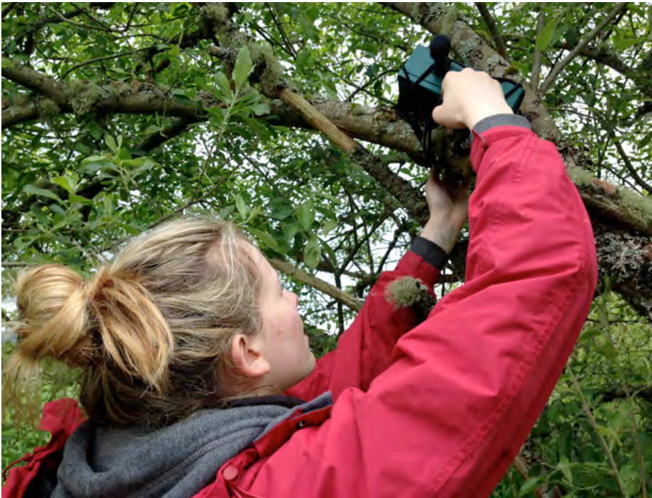
Figure 2. Natalie deploying the passive acoustic recorder at RSPB Loch Lomond (SM2+, Wildlife Acoustics). The recorder is strapped to a branch or stake in a relatively open area overlooking the marsh habitat favoured by water rail.
